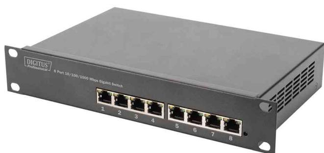
10" Gigabit Ethernet Switch 8 Ports, Vorderseite
